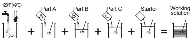
Fill the measuring cylinders for color developers with tempered water. Add color developer part A concentrate and stir to mix developer and water. Add color developer part B concentrate and keep stirring. Add color developer part C concentrate and keep stirring. Add color developer starter concentrate and keep stirring.
